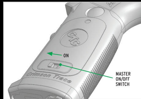
3. SLIDE MASTER SWITCH TO THE FORWARD "ON" POSITION.
